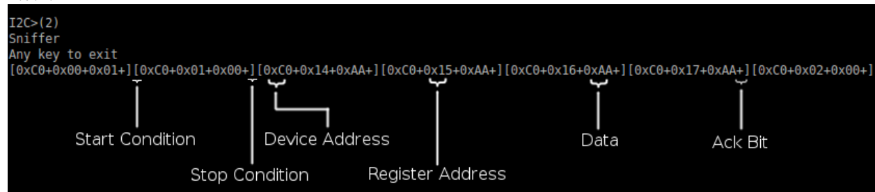
Figure 4.8.1: I 2 C Transaction Between the Microcontroller and LED Driver
